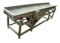
When plenty of water goes into quick-freezing machines, the final quick-frozen products quality will be affected, it is necessary to remove the moisture in the surface of food material, vibration water dropper can remove part of the water in the surface. You can adjust amplitude to control vibration strength. That equipment applies to process soybeans, corn, small peas, and other small granule of fruit and vegetable.
